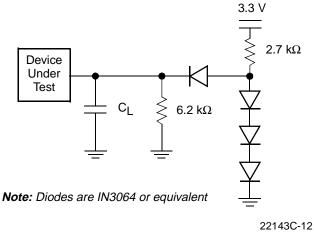
Figure 9. Test Setup
