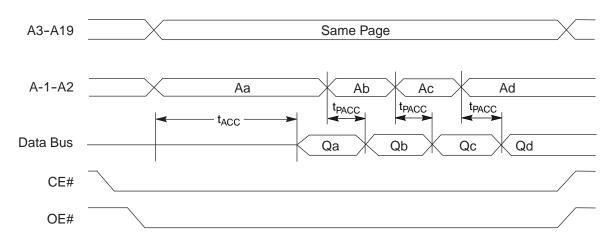
Note: Word Configuration: Toggle A0, A1, A2. Byte Configuration: Toggle A-1, A0, A1, A2.
