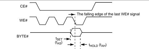
**Note:** Refer to the Erase/Program Operations table for  $t_{AS}$  and  $t_{AH}$  specifications.
