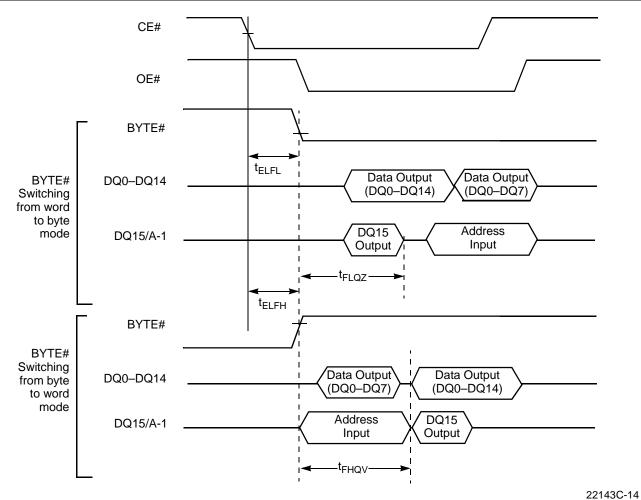
Figure 13. BYTE# Timings for Read Operations
